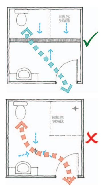
Informative Diagram: Suggested floor waste design for a hobless shower recess within a bathroom to support adequate drainage.
