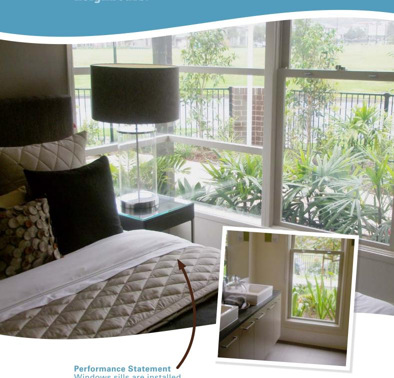
Windows sills are installed at a height that enables home occupants to view the outdoor space from either a seated or standing position.
