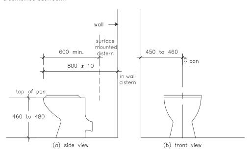
note: for the purpose of dimensioning, the front of the wc pan has been used as the datum plane dimensions in millimetres
