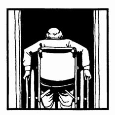
A swinging door is commonly available in a 3' width, but 3' doors are generally used only as front doors on most homes. The usual reason for providing 3' doors is
