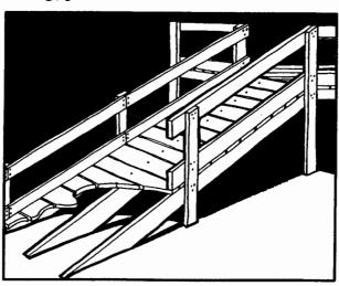
You can also use rolled roofing material. When properly tacked down, it provides a good non-slip surface for walking or wheeling.
