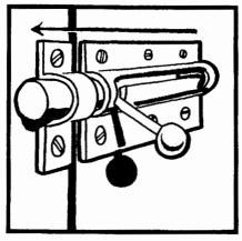
Lever hardware is preferable to any kind of small twist knob. Push buttons may be satisfactory if they don't require find dexterity to release the lock. A push button lock in a cylindrical lever latch is perfect from an operational point of view, but it doesn't generally provide the security of a dead bolt mechanism.
