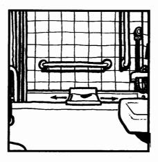
Several types of tub seats are available. Refer to the Resources chapter on page 30 for manufacturers. You can also install a built-in tub seat, which will be more stable and safer than a removable seat. Be sure to carefully design this seat for drainage, so that water runs back into the tub and not out the side when you bathe.
