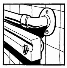
If you make rectangular wooden grab bars, allow closure between the thumb and fingers of your hand. This provides the best grip when you close your hand around the bar. The optimum diameter for grab bars is 11/4-11/2" for adults. For a child or person with a very small hand, the ideal diameter is 1-11/4". The distance between the wall and the grab bar should be 1½". A wider space can be dangerous if you slip and your elbow lodges between the wall and the bar. A narrower
