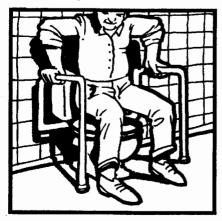
The sheltering arm grab bar surrounds you, providing support similar to the arm rest of a standard chair. It allows you to use your arm and leg muscles to lower yourself onto the toilet and return to a standing position. Sheltering arms also provide better balance support while you are seated on the toilet.
