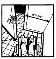
Unfortunately, to enlarge a landing you may have to relocate walls or partitions. This may be a difficult task, especially in older homes where walls or partitions bear the weight of the house or where electrical or plumbing lines are located.
